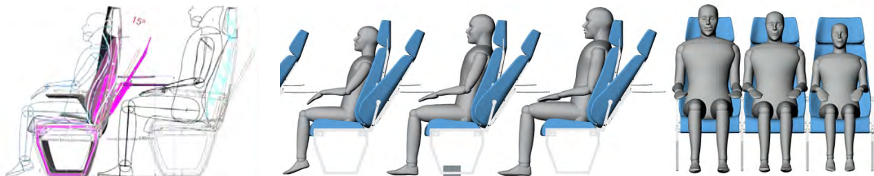
Figure 2: Virtual model ergonomic verification with seat structure 15°
