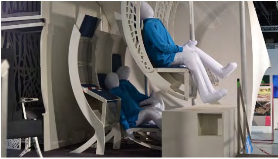
Figure 1: The chaise longue seat of the Flying V using the vertical space in the aircraft cabin.
