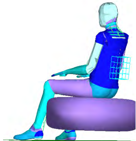
Figure 1 : Human model in vibration test on experimental seat with configurable backrest with foam block modelled using finite elements.
