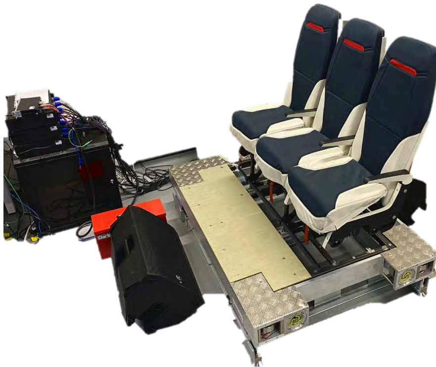
Fig. 1. Aircraft seat mounted on a vibration simulator. The centre seat was used in the study. The image also shows amplifiers and positioning of loudspeakers.
