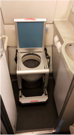
Figure 4: Hamburg On-board Wheelchair Prototype in A320 lavatory
