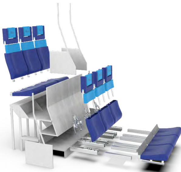
Figure 2: Exploded view of 6 seats indicating its modularity. The seat pan of the lower row can disappear under the back rest enabling in- and egress.
