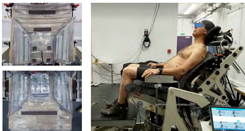
Figure 1. Location of the inflatable air cushions on the seat pan and backrest (on the left) and an overview of the experimental set-up with a participant
